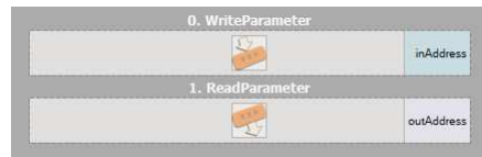
Global parameter "inAddress" created within the filter WriteParameter can be read with the ReadParameter filter.
